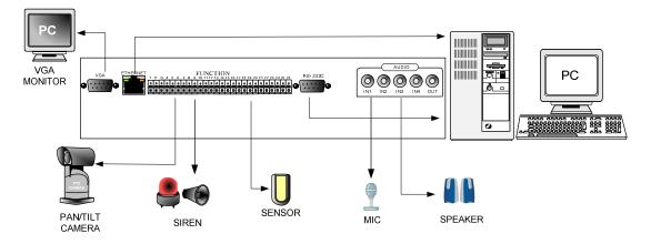
**RS-232C** : Control DVR through RS-232C port by using PC.
